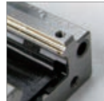
Inspection intervals 1 and 2: Lubrication Maintained
