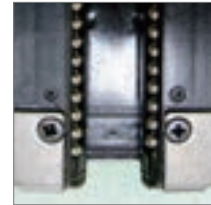
Plastic parts and end seal in good condition
