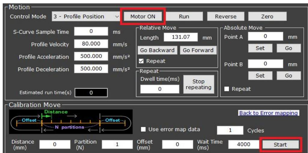
The motor will then move to the user-assigned-position to start measuring (see Ch. 4.9.2, point #2) and perform the Calibration Move.
