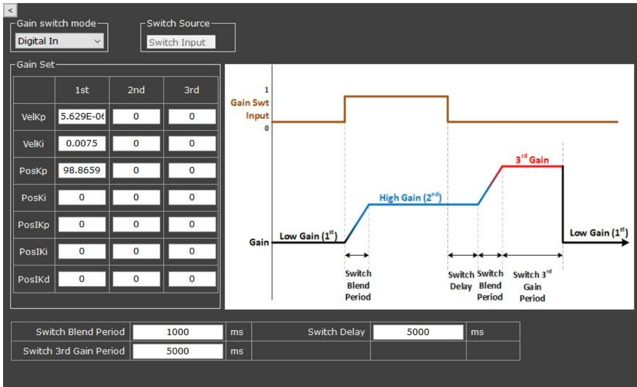
Use digital signal input to determine which gain-set to be applied.
