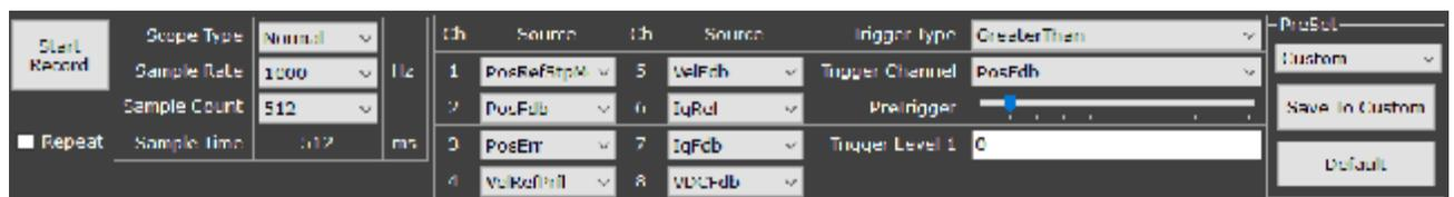
Like using an oscilloscope, users need to set up first the scope type, rate, sample count, and the data (channel number and the source).
