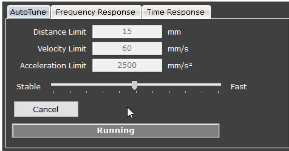
The motor will move back and forth while tuning velocity. Set the moving distance limit and click “Tune” button, the UI will tune the velocity loop gain automatically.
