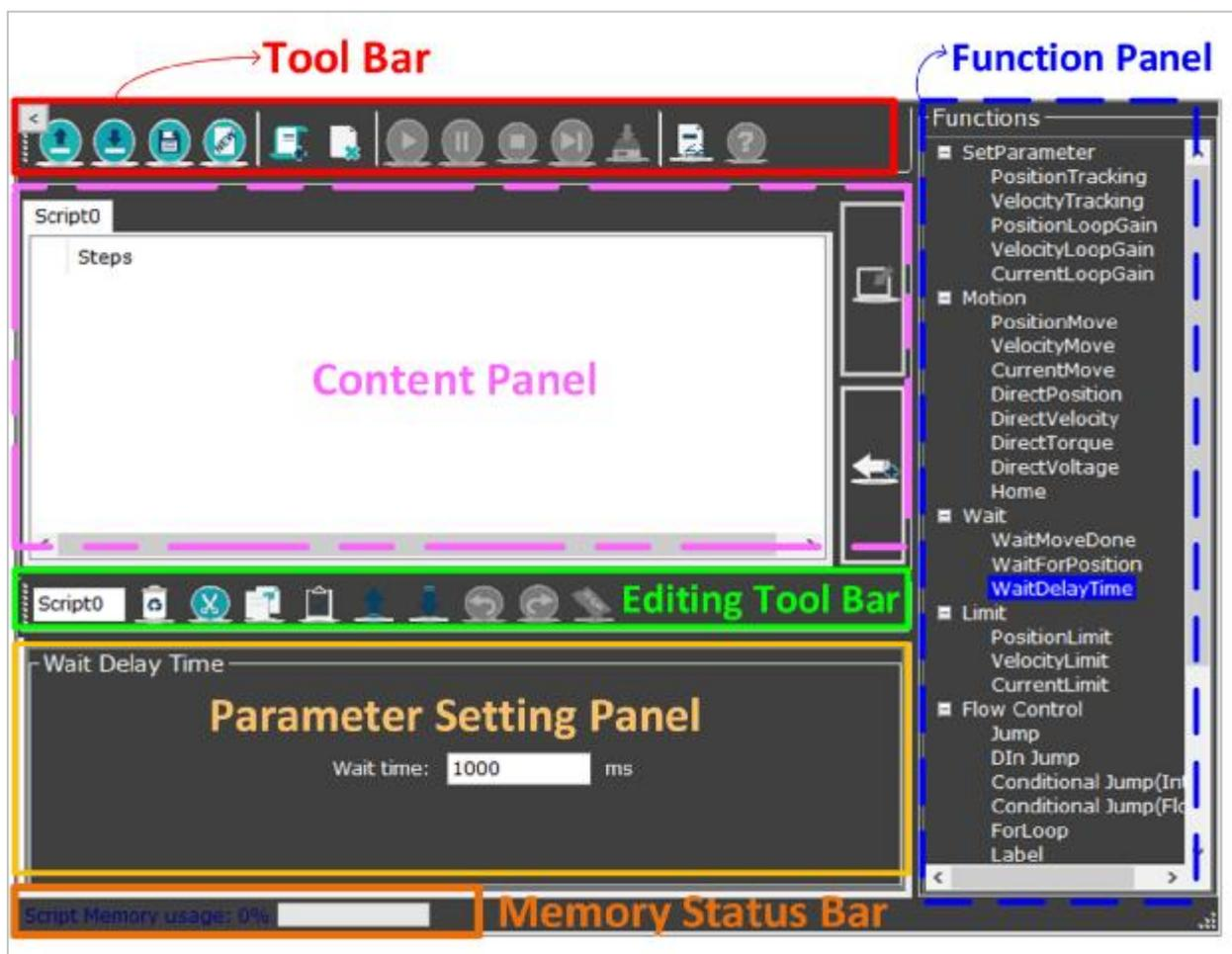
1. Tool Bar – on top of the interface, for processing file and executing script.
