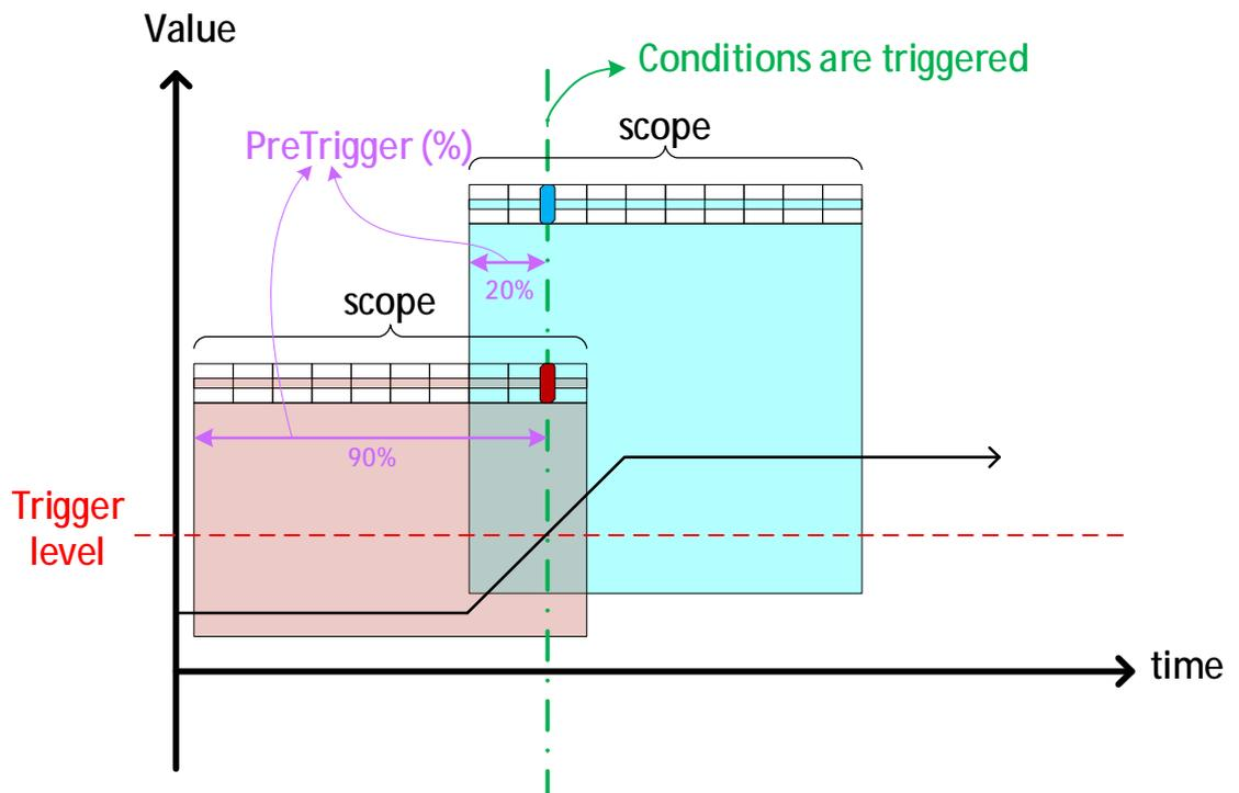
The scope on the left is with PreTrigger 90%, meaning that 90% of the data shown on the *left* scope is below trigger condition(s). Likewise, for the scope on the *right*, 20% of the data shown on the *right* scope is below trigger condition(s)
