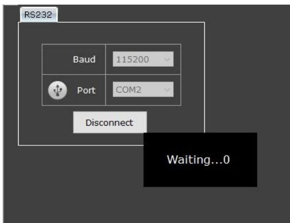
3. When the columns turn grey, it means the driver and the host computer are successfully connected.
