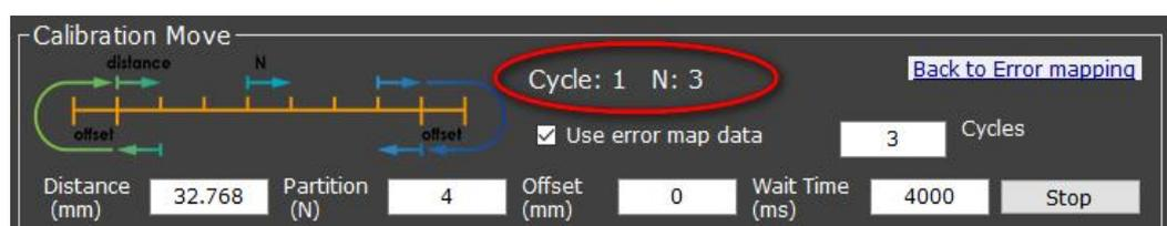
4. After calibration move(s) are finished, click [Back to Error mapping](#) button.
