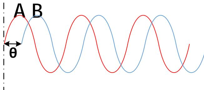
The sine and cosine signals can be drawn into a circle based on X (sine) and Y (cosine) co-ordinates and can therefore perform arctangent function (or, interpolation) to know the degree of theta in order to obtain finer position resolution.
