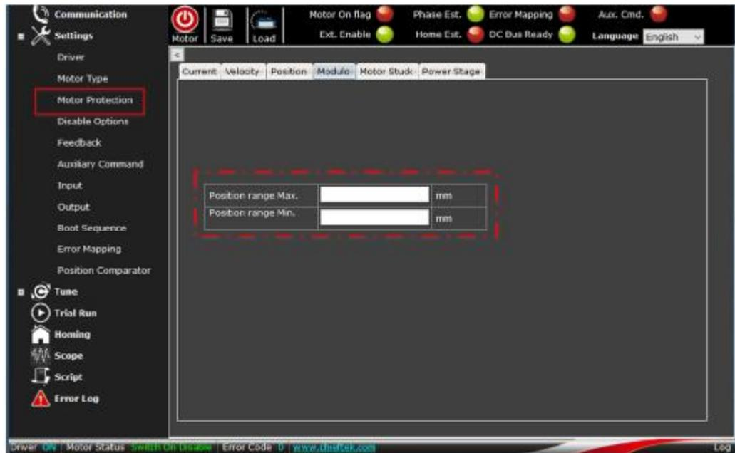
2. This major rule applies to all combinations of motor type, motor mode, and position command type: **If position command exceeds or is lower than the Position Limit, this command will be ignored.**
