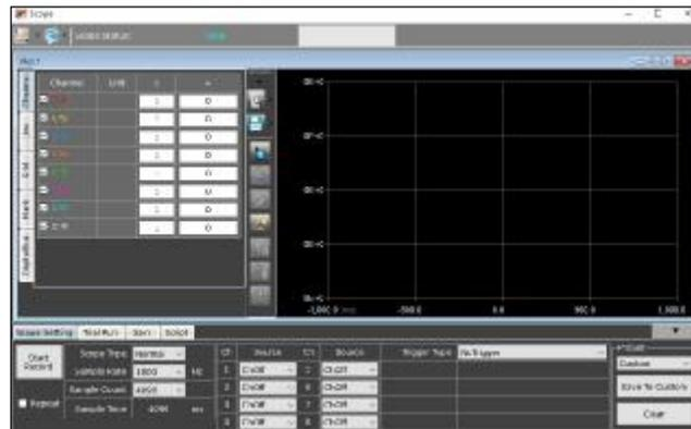
3. In Scope, set the source of channel 1 to ThetaElec and the source of channel 2 to Hallcode. Next, select “Normal” for Scope Type (see picture in step 4).
