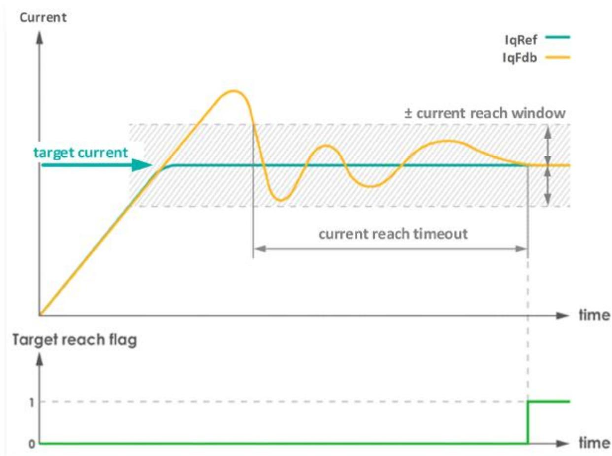
$I_{qFdb}$  refers to current feedback; likewise, velocity applies the same method to rise target reach flag and to determine whether the reference command is met.
