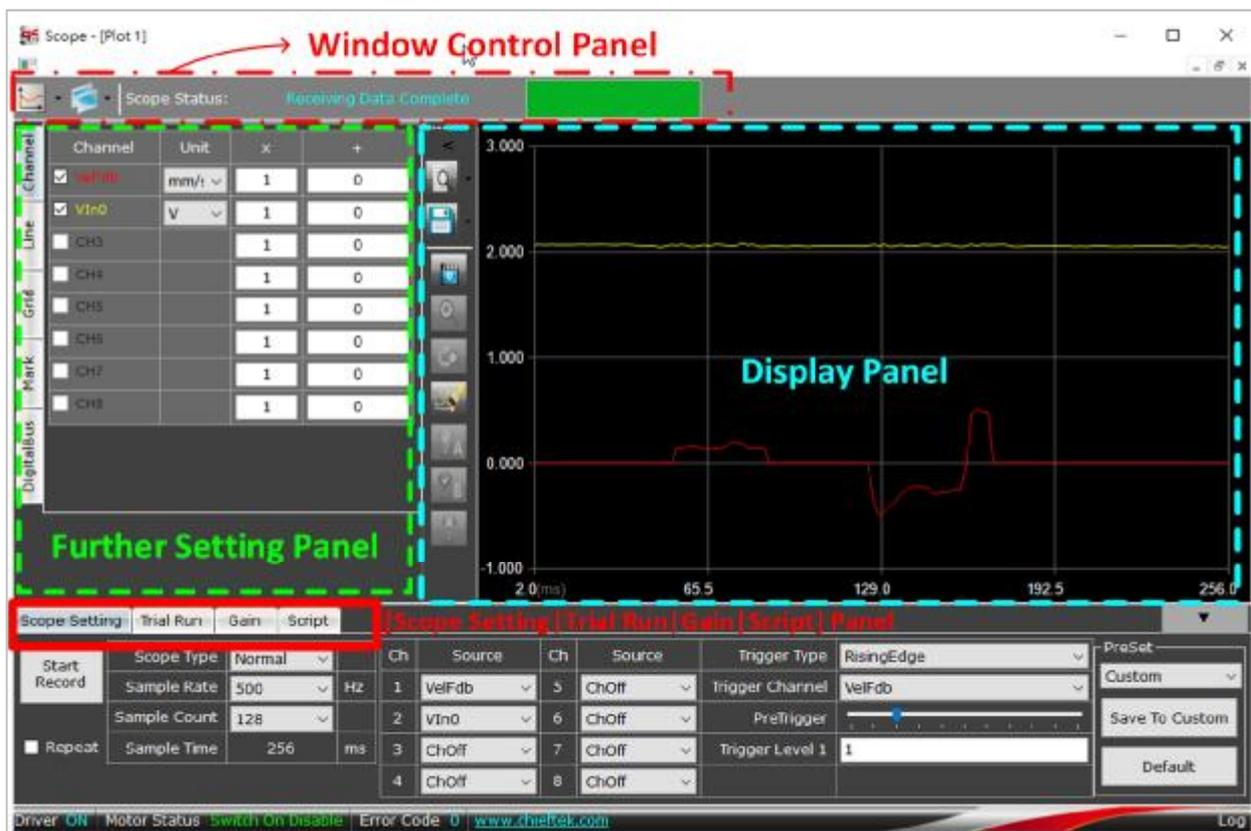
You can use Scope to monitor several variables by setting them as the channels' data source (see chapter 6.1). Also, you can configure the data unit and graph details. Moreover, Scope allows you to record data and alter the data presentation way.
