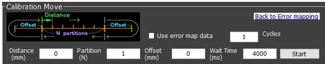
This panel is a convenient tool for designing a set of consecutive motor movements to work with a finer device.
