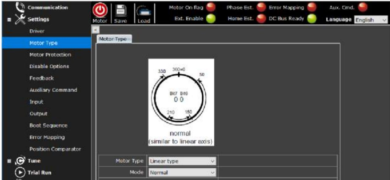
The “Motor Type and Mode” table below shows each motor-mode’s effect on Position Limit (i.e., Command Forward/Backward Limit) and Position Range (i.e., modulo); see explanations on next page. The following chapters elaborate on details of these 6 type-mode combinations.
