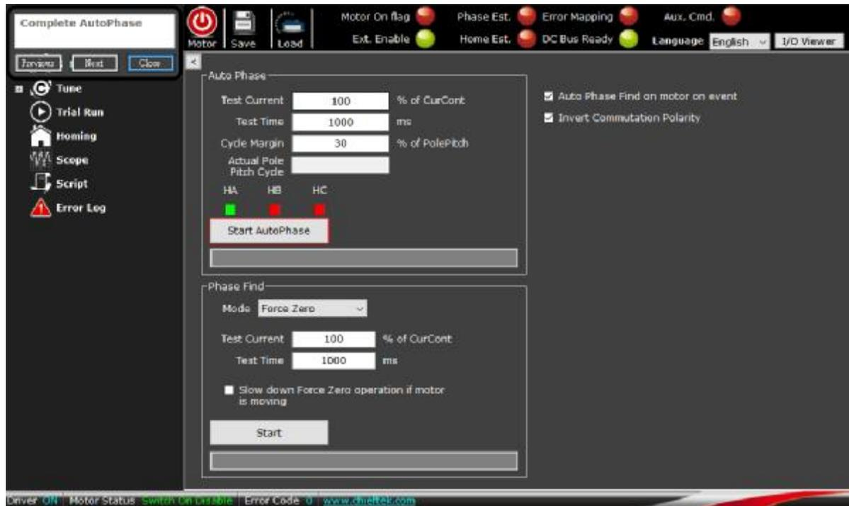
2. Move the motor manually at least one pole pitch in positive direction.
