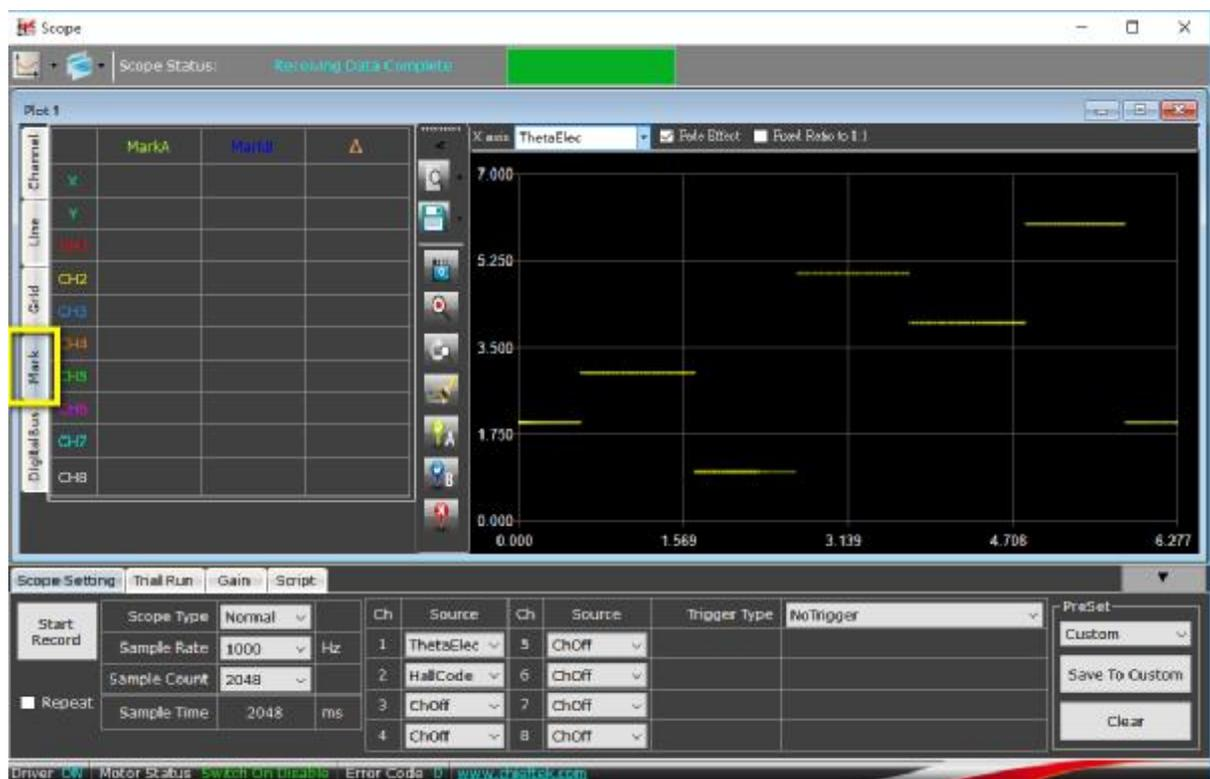
8. Click on the Mark A icon
