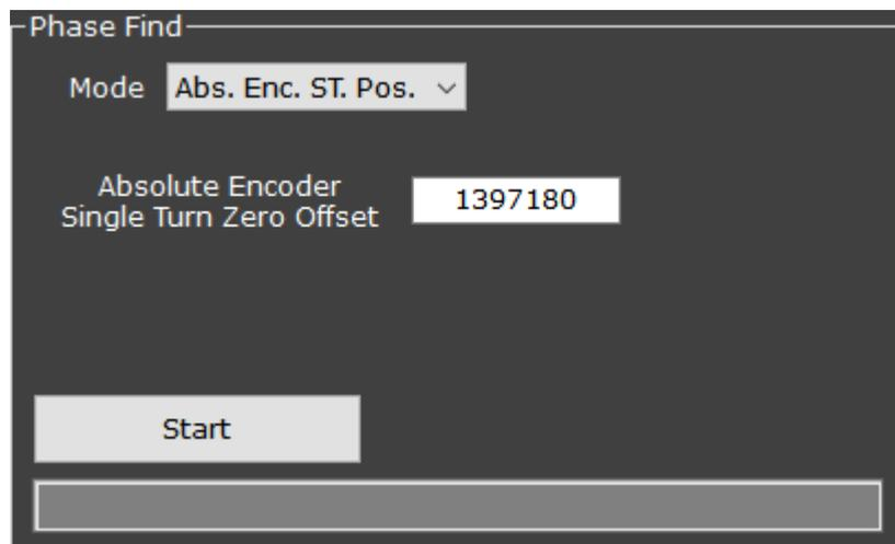
To operate with an absolute encoder, execute AutoPhase first in order to initially locate what position count corresponds to “0” electric angle (i.e. theta value 0)—this position count value is the “Absolute Encoder Single Turn Zero Offset” value.
