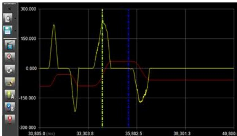
The information **MarkA** **MarkB** and differences **Δ** between marks A and B are shown on the “Mark Tab” of Further Setting Panel.
