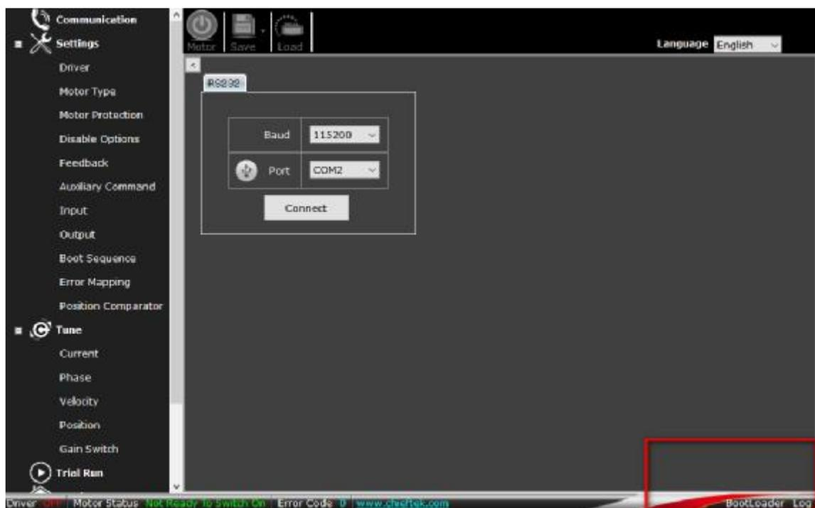
5. The Boot Loader interface will jump out automatically.
