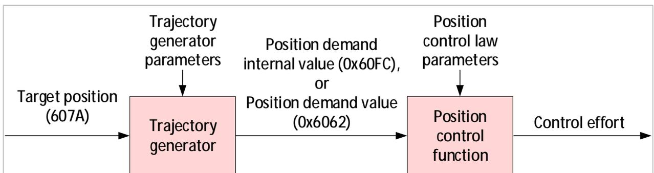
At the input to the trajectory generator, parameters are limited before being normalized to the internal units.
