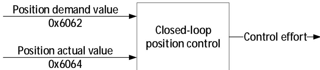
To make sure that the physical limits of a driver is not exceeded, an absolute function is implemented – the current limit function and the velocity limit function – for the position control effort.
